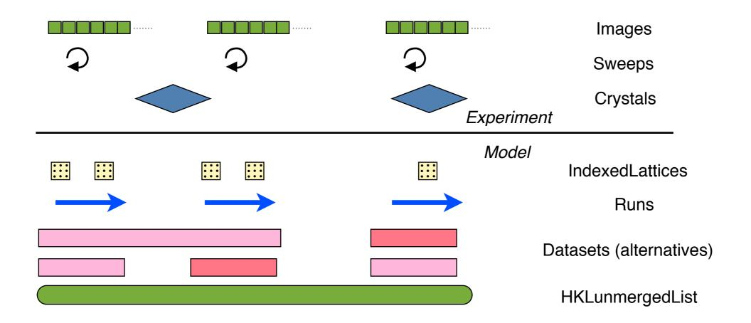
Top 3 classes describe the experiment: put crystal in beam, rotate, collect contiguous images A *IndexedLattice* is an indexing, with cell, orientation, and (ultimately) space group *Run* is just a list of lattices for a sweep
